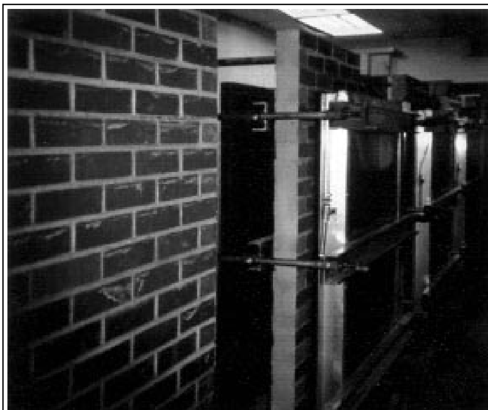
Water Penetration Walls, Ready For Test
