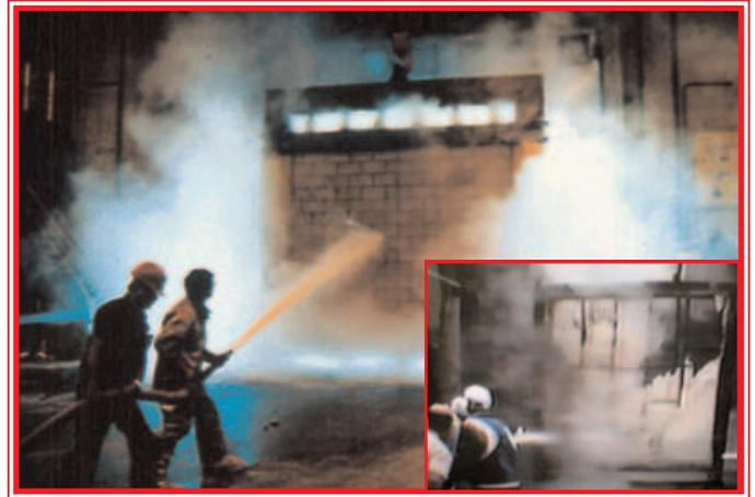
CMU sample passes the hose stream test. While the Panel-and-stud assembly (Inset) virtually disintegrates.
