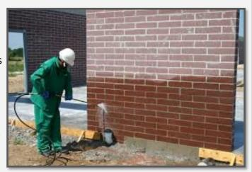
that no rain water would penetrate the wall and cause efflorescence.
