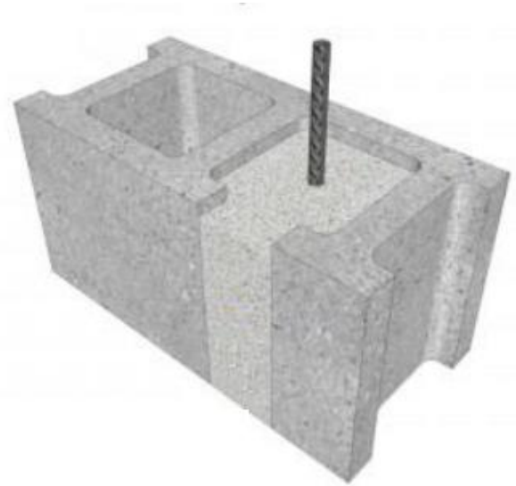
Figure 2: Sawcut existing masonry core and insert vertical rebar. Grout flush to adjacent faceshells. (Note: grout filling at the installation of horizontal rebar will be similar) Source: IMI Masonry Detail Series
