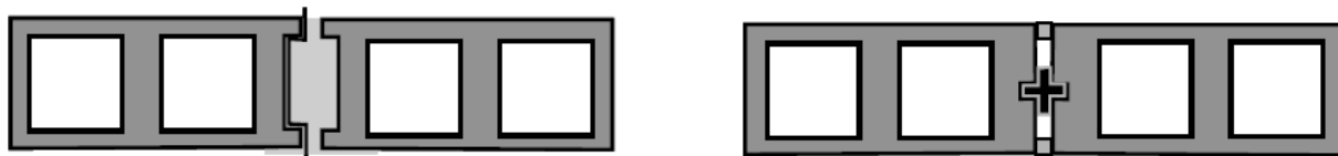
Figure 1: Shrinkage Control Joints (From Klingner 2010)
