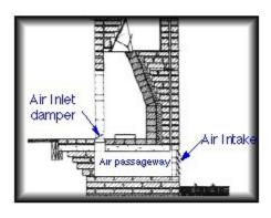
The other figures on the chart show the increased efficiency of using an air circulation insert. These are steel boxes that are inserted into the masonry fireplace which allow air to be heated and then use a fan to circulate heated air back into the room. There are many manufacturers of these products available on the market which can enhance the efficiency of a fireplace.
