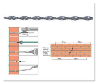
A great use of helical ties is in stabilizing masonry structures in earthquake prone areas. Other uses are in stabilizing parapets, anchoring stone, terracotta, stucco and replacing wall ties when masons use wall ties in areas that are not just wood stud backup.
