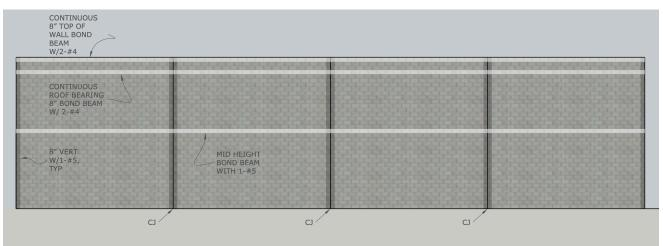
These examples show the options for horizontal reinforcement with regular CJ locations. There are situations when regular CJ are either not possible or not desirable for a variety of reasons.
