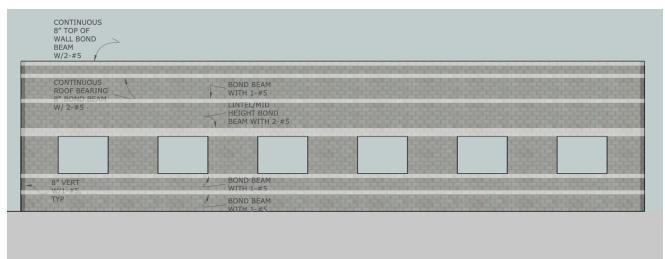
**5** OPTION 5: BOND BEAMS AT 48" O.C. WITH NO CJ Scale: 1/8" : 1'-0" Finally, using the criteria we have defined above, we also have another option in masonry walls with both horizontal joint reinforcement and bond beams. One example of when this may occur is for masonry walls that are the back up wall and part of a cavity wall system. When the brick is anchored to the backup wall utilizing the joint reinforcement. In this scenario, the bond beams can be spaced further apart.
