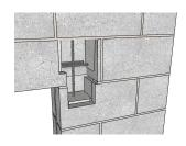
**Third**, the masonry wall CJ's should be located away from openings. Masonry lintels create an integral joint with vertical jamb reinforcement. This leads to a more robust design that has many analysis and design benefits including arching action and fully developed lintel reinforcement. For more information of CJ placement, see NCMATEK 10-2D at https://ncma.org/resource/tek-index/
